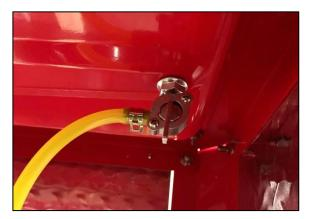
To start the engine place the "Main Tank Fuel Valve" in position shown (left).
