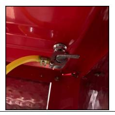
Placed on the top of the main tank is the sticker stating "<u>FUEL SHUT-OFF UNDER TANK</u>" Located directly under this sticker is the <u>Main Tank Fuel Valve</u>, one of the three fuel valves. Above right picture showing valve in the "<u>Off Position</u>". (Handle to horizontal right position.)
