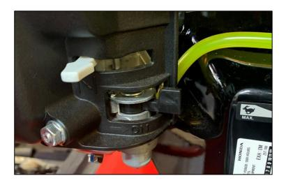
Pictured left is the factory Choke lever (White) and Fuel Lever (Black), this valve is the third of the three fuel valves.
